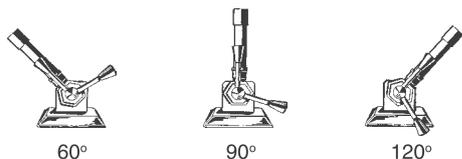
To adjust the burner to the angle which suits you the best, simply lift it out of its base and reinsert it in the required position. The burner is thus equally well suited for left-handed and right-handed users.
