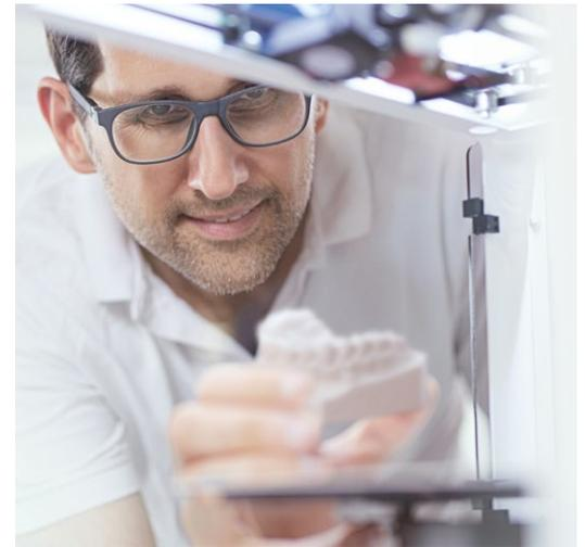
parameters for each model? Because the diagnostic model should primarily have a clean, white appearance, while the wall thickness of the working model must be designed so that it can also withstand 2.5 bar in the pressure pot. The thermoformed aligner model, in contrast, must be heat-resistant.
