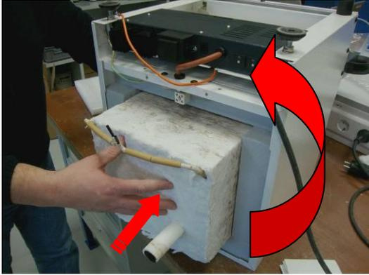
Fig. 41 – Installation of new muffle
